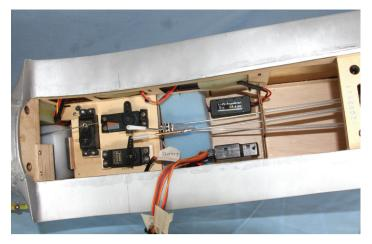
A neat radio installation, but I had to extend the rudder pushrod (see text)
