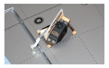
A standard size servo fits neatly into the aileron servo box
