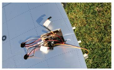
Three servo leads from each wing panel to be connected; note the central retract servo
