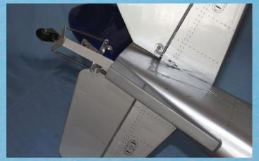
Steering tailwheel assists ground control; note the scale moulded covering over the tailwheel bracket
