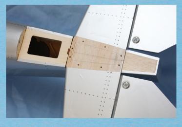
Remove film covering from this area to adhere the fin seat
