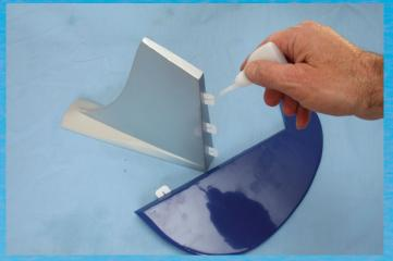
Thin cyano will hold the slotted Mylar hinges for the control surfaces
