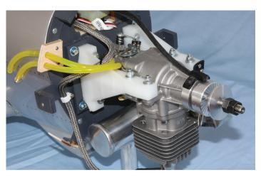
The powerplant chosen was the DLE 20 cc petrol, which required a little modification to the firewall but the space inside the cowl is ample
